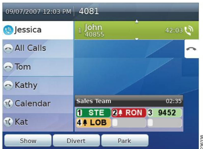
Figure 23: CiscoIPPhoneStatusFile Object Display Sample
